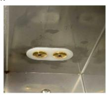
If there is no water being sensed and the water is determined to have proper mineral content for conductivity then it is possible that one of the wires on the back side of the assembly has been disconnected.
