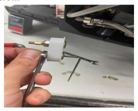
Note: the assembly has tension springs which will cause the contactor screws to push inward when seating the reservoir. It is important to ensure that the threaded posts are not touching the white housing during reassembly as this can cause the post to hang up and stay seated back away from the reservoir.
